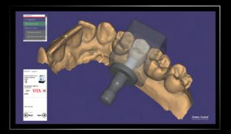
With the help of exocad ChairsideCAD, crowns, inlays, onlays, veneers and small bridges can be designed and manufactured directly at the treatment center in a very innovative and fast workflow. Using the integrated In-CAD Nesting module, the designed jobs can be placed directly in the block for calculating and milling by the machine.
